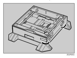
Adjust the four corners of the printer to those of the 500sheet paper feed unit, and then lower the printer slowly into place.
